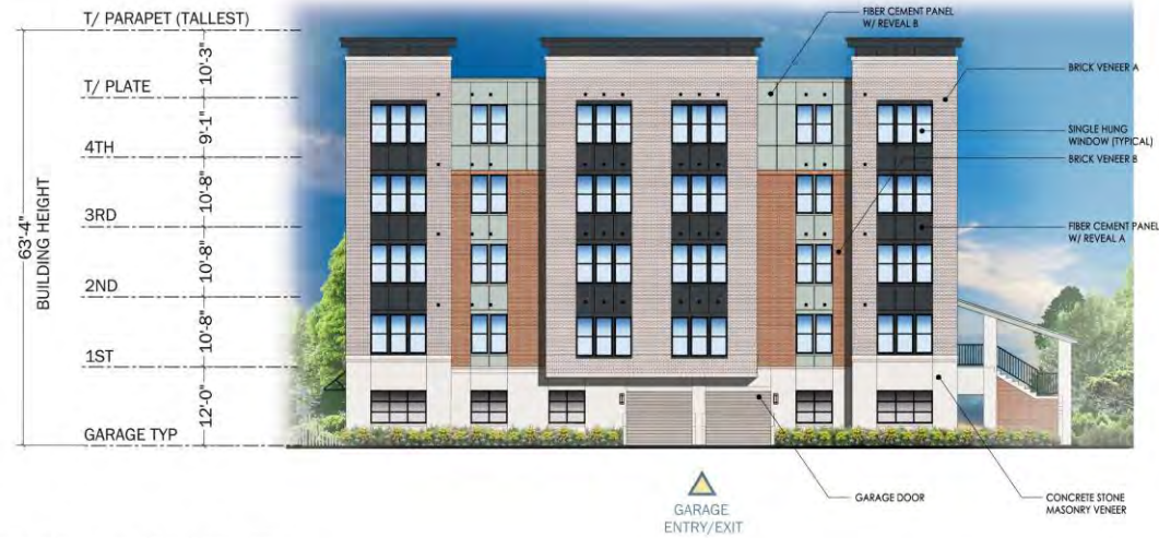
02 - SIDE ELEVATION (GARAGE ENTRY)
